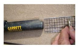
I tested (tried to test) the depth ability of the 3 pinpointers on 4 separate occasions. The results were discouragingly inconsistent, both during each test, and as compared to other tests. Never-the-less, it appears the White's TRX obtained more depth than either of the Garrett's, but this advantage can be mitigated to a widely varying degree by using the Garrett Coin Slide. This is a neat little trick most of the
